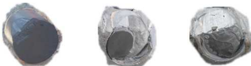
(a) Mechanical fatigue failure (b) Crack failure (c) Delamination failure
