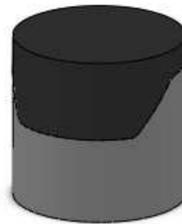
Fig.5 Solid model of Multi-face PDC cutter
